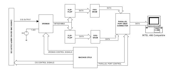
Figure 1. Block Diagram of XRD9829REF
